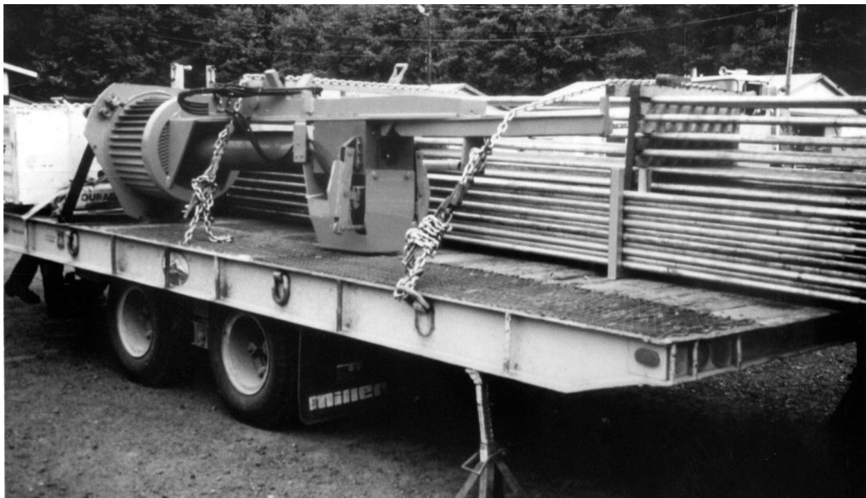
Photo 1. Soil nail launcher and nails ready for transport (USFS, 1994).
